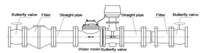
$\star$ Before using this water meter, the pipe must be filled with water, otherwise it will lead to inaccurate or even non-measurement.
